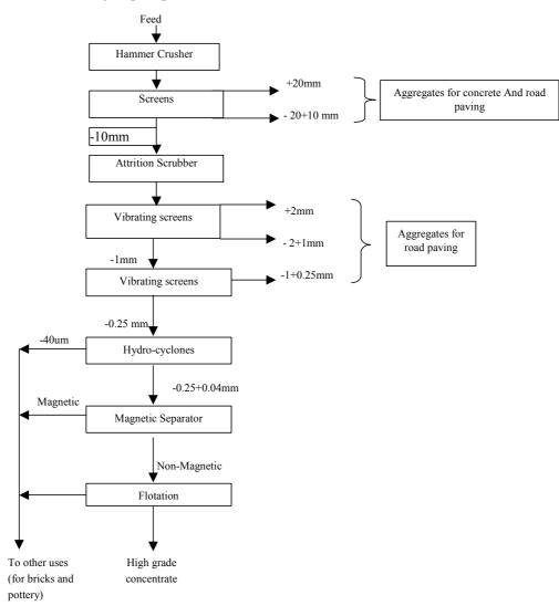
Fig.2. Proposed flow sheet for flotation of Sebaeya low grade phosphate
